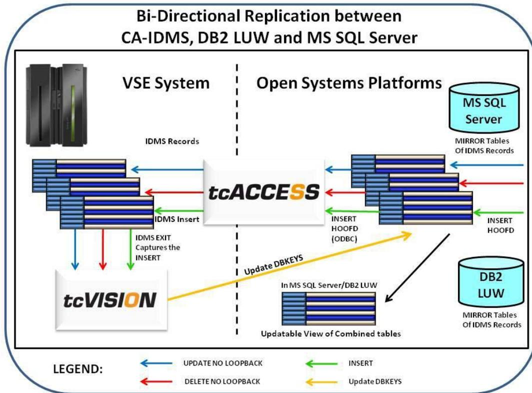
The diagram shows the bi-directional synchronization between the VSE CA-IDMS database and various Unix and Windows applications that store their data in DB2 LUW and MS SQL Server databases.
